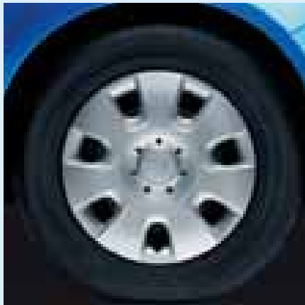
5.0J x 14" steel wheels for 175/70 R14 tyres with Draco hub covers.
