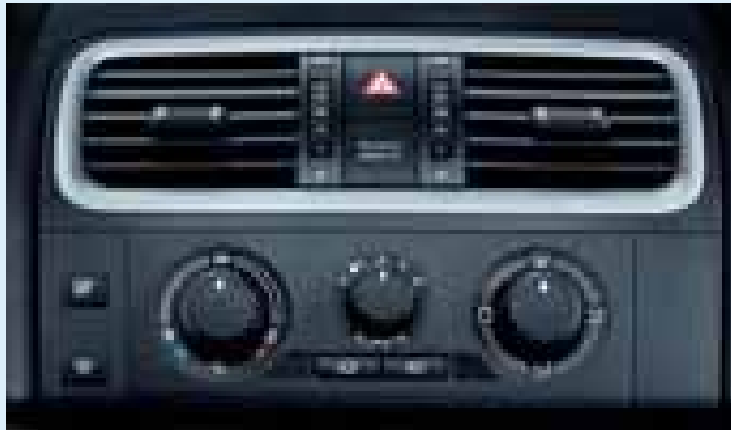
Semi-automatic air conditioning system Climatic: automatic maintenance of preset temperature of the air inflow, manual regulation of air volume and setting of exhaust.
